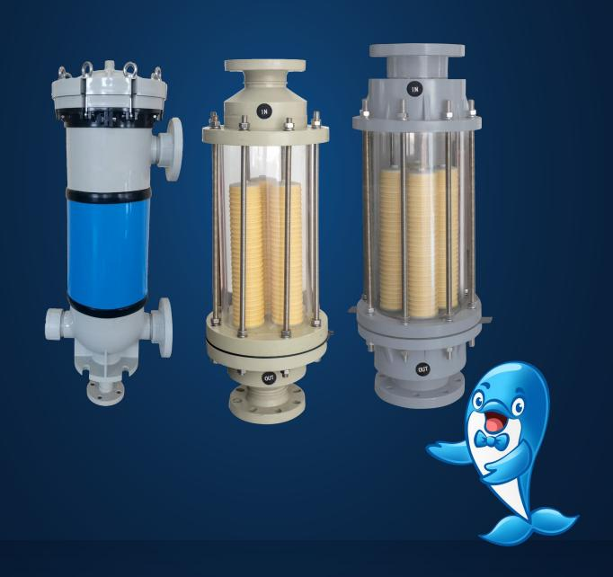
The Resin Trap is mainly installed on the water system pipeline at the outlet of equipment containing resin such as ion exchangers. When the nozzle or the water distributor are damaged, resulting in the leakage of resin passing through, it can be intercepted and captured by the Resin Trap to avoid affecting the downstream system.
