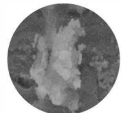
Aragonite type (soft and amorphous, easy to fall off and clean)
